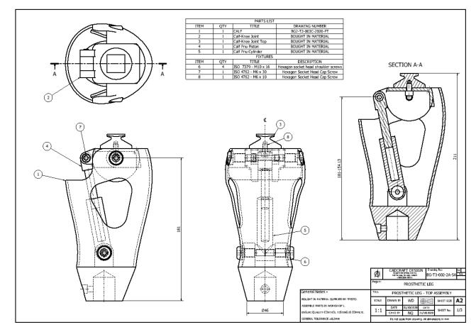
Assignment 2B: PROSTHETIC LEG BOTTOM ASSEMBLY
